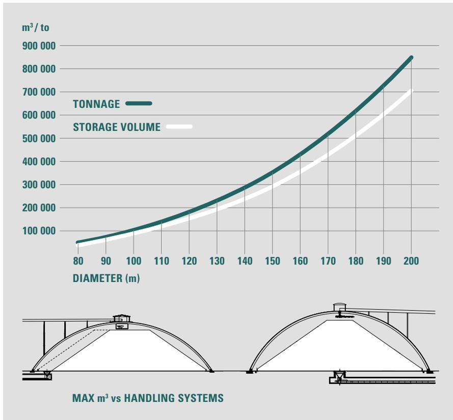
**BULK DEFINE SPECIFICATIONS** \_Angle, density, input and output feeding, stock method for your operating equipment. Our Dome handling operations solution allows you to achieve the full benefits as part of an optimized package.
